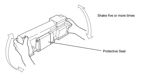
6. Carefully remove the protective seal.
